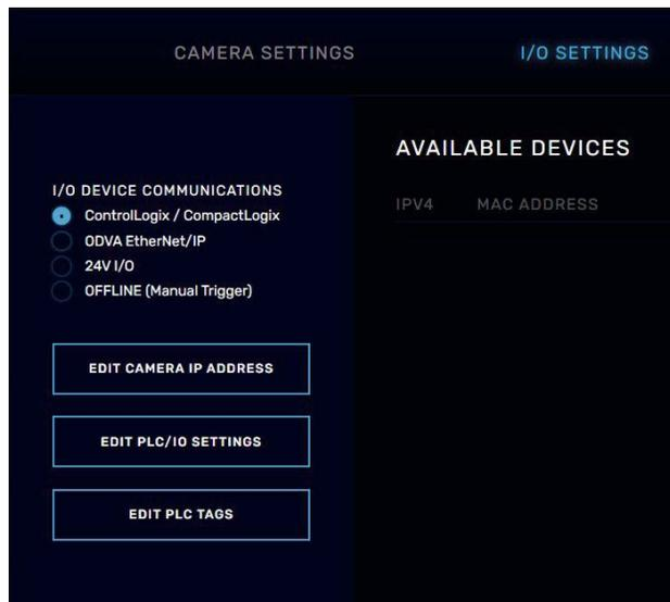
**Note:** Write down the new IP address before applying changes. Changing the subnet will **disconnect the camera**. You must **update your PC's subnet** to match the camera's new network (see **Page 5** for instructions)
