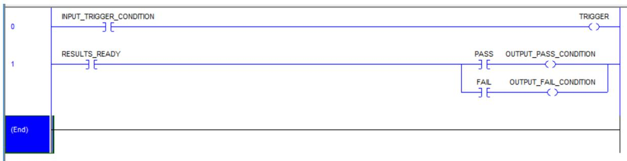
**Note:** Each time **TRIGGER** is set high, **RESULTS\_READY**, **PASS**, and **FAIL** are reset to low.
